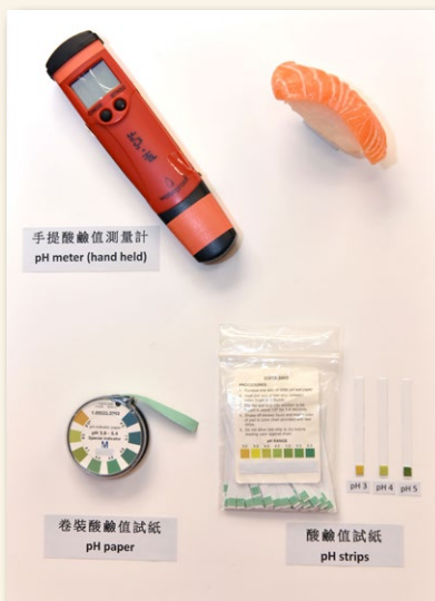
一些測量壽司飯酸鹼度的工具 Some tools for measuring pH of sushi rice
