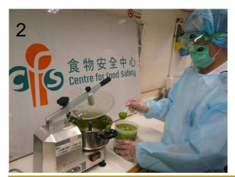
Prepare sample for screening in the Contamination Monitoring System (CMS)
